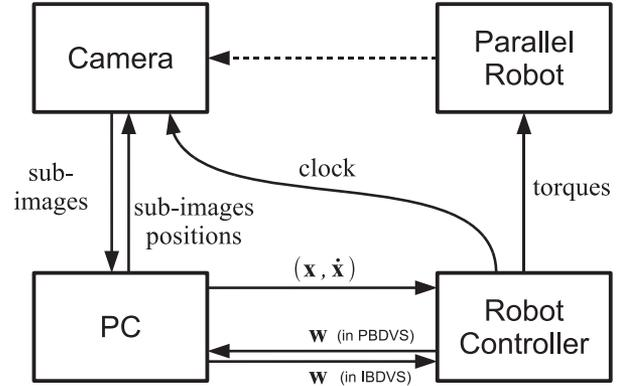
**Fig. 7.** Data flow in the implemented control architecture. In PBDVS the pseudo-control vector  $\mathbf{w}$  is computed by the DSP card and transmitted to the PC to improve pose and velocity estimation while in IBDVS  $\mathbf{w}$  is directly computed in the PC and transmitted to the robot controller.
