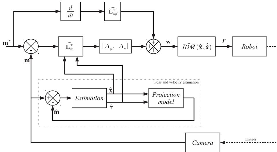
**Fig. 5.** Image-based dynamic visual servoing. The pseudo-control vector (acceleration) is computed from visual features. Pose and velocity estimation is provided thanks to the method presented in Section 2.
