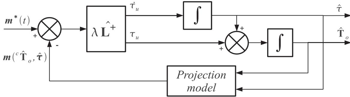
Fig. 2. Pose and velocity estimation under constant velocity assumption, using the virtual visual servoing paradigm.
