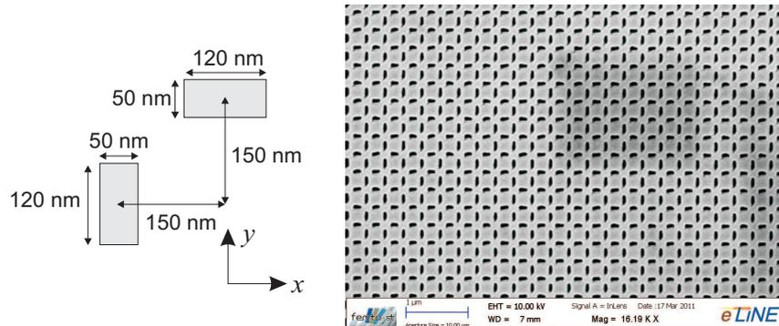
Fig. 1: Scheme of one period of the sample and SEM image of one of the fabricated samples on a 100 nm thick gold layer.
