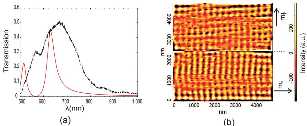
Fig. 2: (a) Experimental (dotted line) and theoretical (solid line) transmission spectra through the sample and (b) near-field image obtained with a SNOM working in transmission mode @ 633 nm. The incident polarization is horizontal in the bottom of the image and vertical in the upper part.
