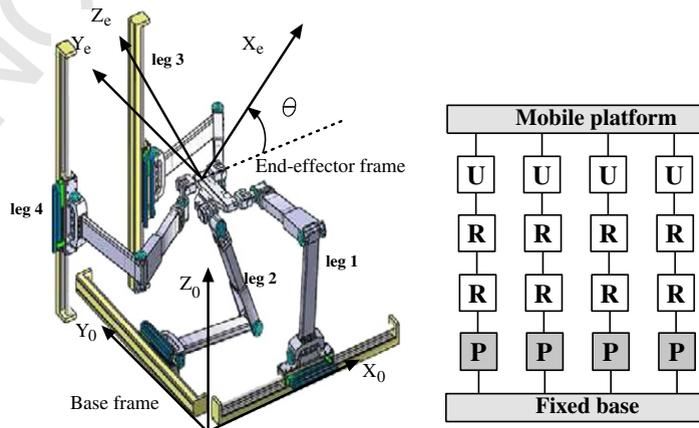
Fig. 4. Structure of the Isoglide4-T3R1 (left) and its kinematic scheme (right).
