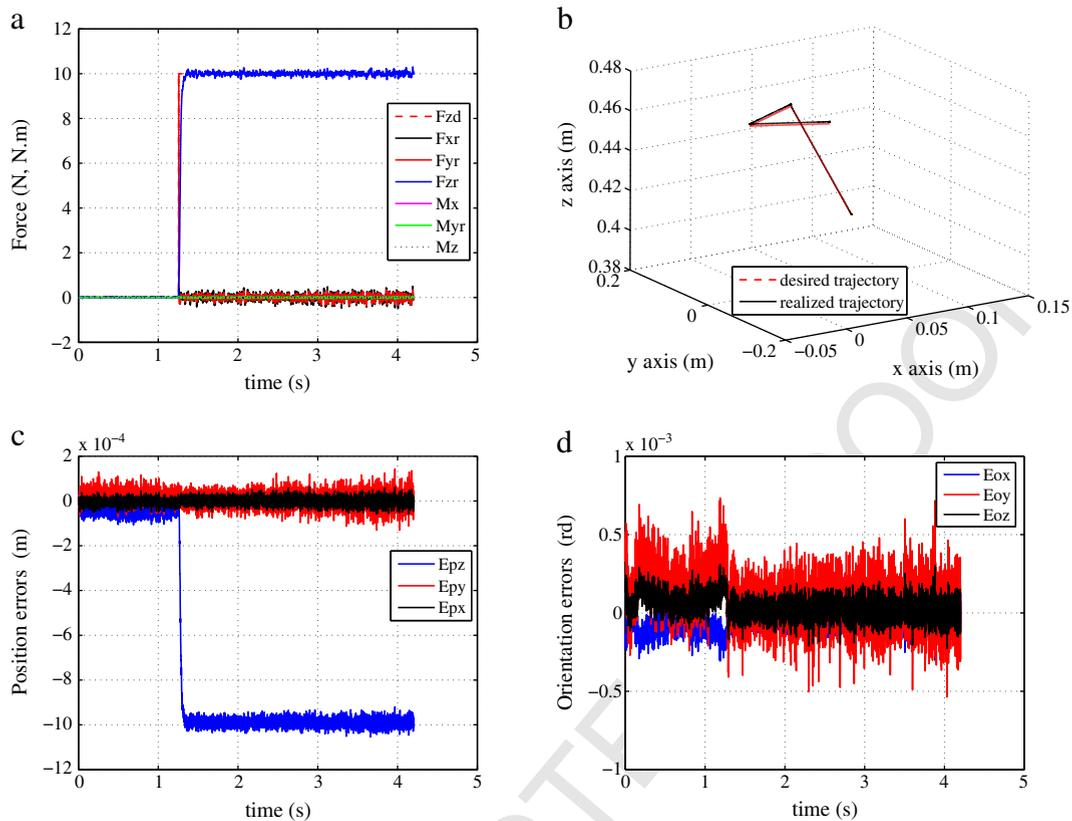
**Fig. 15.** Results obtained with the Gough–Stewart robot in Case 1: (a) Desired and realized forces, (b) 3D Cartesian trajectory, (c) Cartesian position errors, (d) Cartesian orientation errors.
