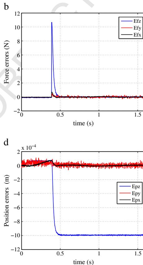
Fig. 10. Results obtained with the Orthoglide in Case 4: (b) force errors, (d) Cartesian position errors.
