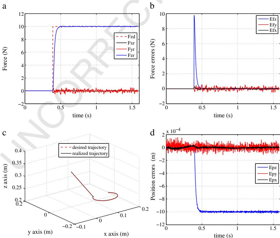
Fig. 7. Results obtained with the Orthoglide in Case 1: (a) Desired and realized forces, (b) force errors, (c) 3D Cartesian trajectory, (d) Cartesian position errors.
