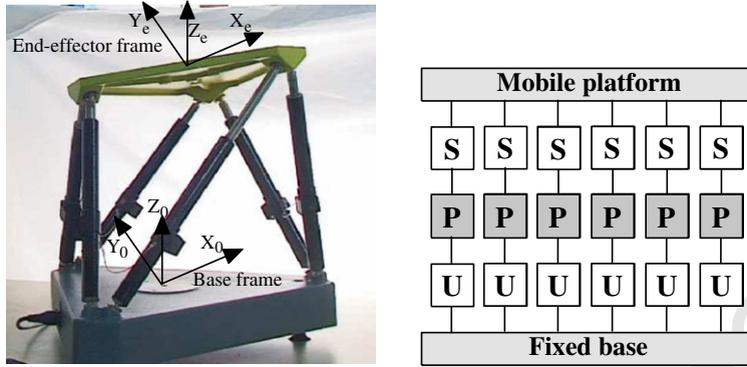
Fig. 5. A pedagogic implementation of the Gough–Stewart platform (left) and its kinematic scheme (right).
