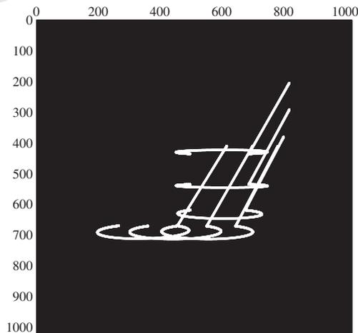
Fig. 6. Projection of the Orthoglide desired trajectory in the image plane using a 6 blob visual pattern.
