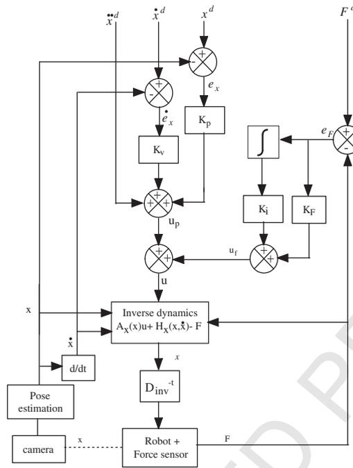
Fig. 2. The proposed parallel vision/force control.
