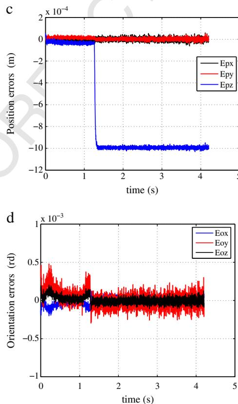
Fig. 16. Results obtained with the Gough–Stewart robot in Case 2: (c) Cartesian position errors, (d) Cartesian orientation errors.
