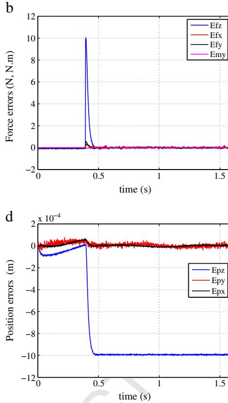
Fig. 14. Results obtained with the Isoglide in Case 4: (b) force errors, (d) Cartesian position errors.
