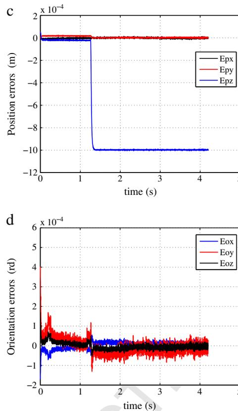
Fig. 17. Results obtained with the Gough–Stewart robot in Case 3: (c) Cartesian position errors, (d) Cartesian orientation errors.
