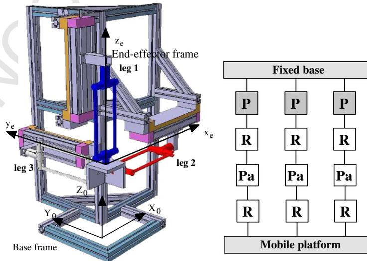
Fig. 3. Global view of the Orthoglide (left) and its kinematic scheme (right).
