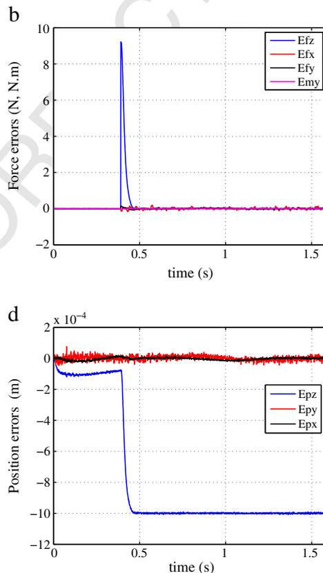
Fig. 12. Results obtained with the Isoglide in Case 2: (b) force errors, (d) Cartesian position errors.
