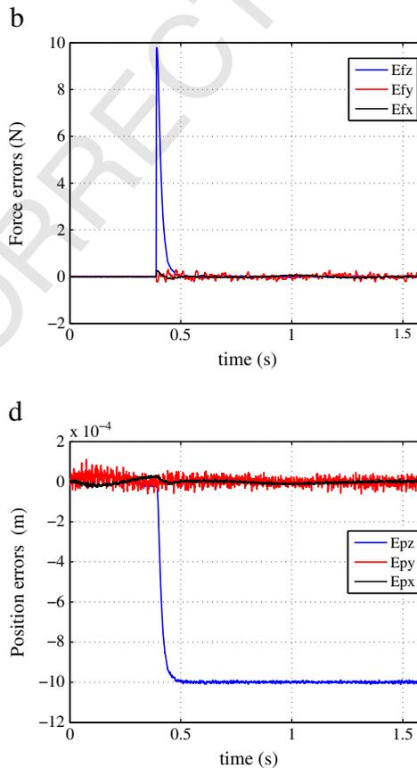
Fig. 8. Results obtained with the Orthoglide in Case 2: (b) force errors, (d) Cartesian position errors.
