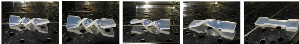
Figure 2: Shape memory demonstration of the Veriflex ® , the specimen autonomously returns to its original permanent shape when heated at 120 °C.
