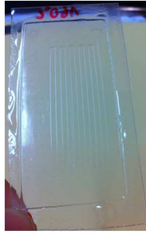
Fig. 20. Roll embossed micro-fluidic devices.
