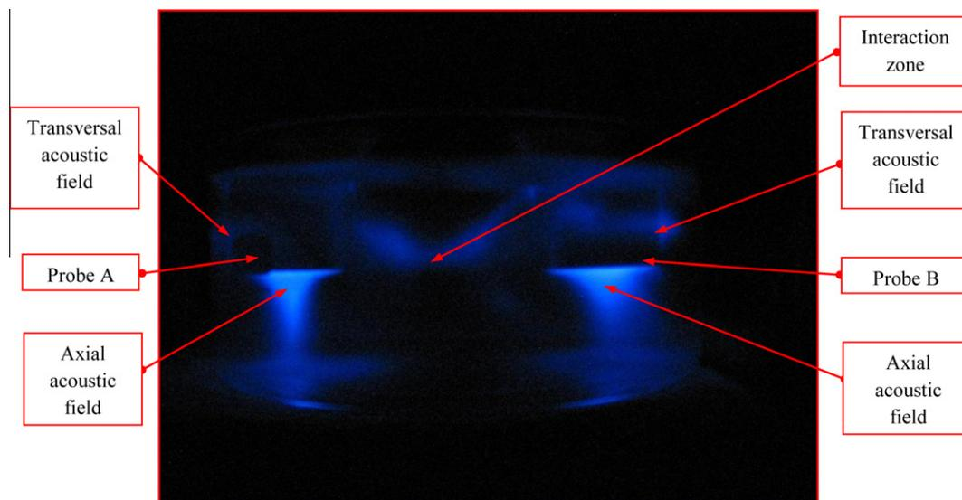
Fig. 4. Photography of sonochemiluminescence for two devices running together.
