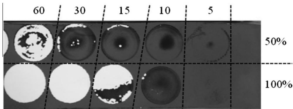
Fig. 6. Static cleaning and etching test on auto-polishing painting with two wave amplitudes (50% and 100%) and five sonication times (5–60 s).
