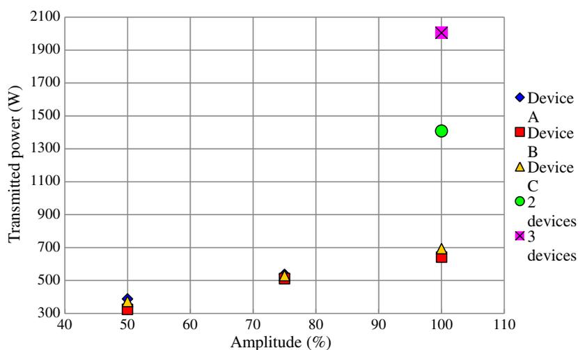
Fig. 3. Transmitted power versus amplitude for single or multi devices.
