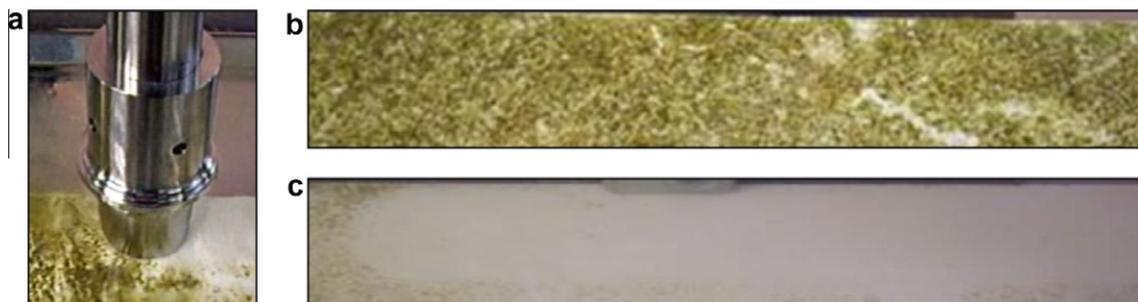
Fig. 5. Dynamic cleaning test of a dirty sample: a. Ultrasonic device cleaning the sample; b. dirty sample before cleaning test; c. dirty sample after cleaning test.
