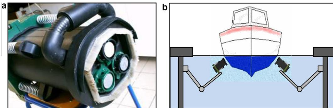
Fig. 2. Cleaning tool: a. Photograph; b. cleaning station with two devices.
