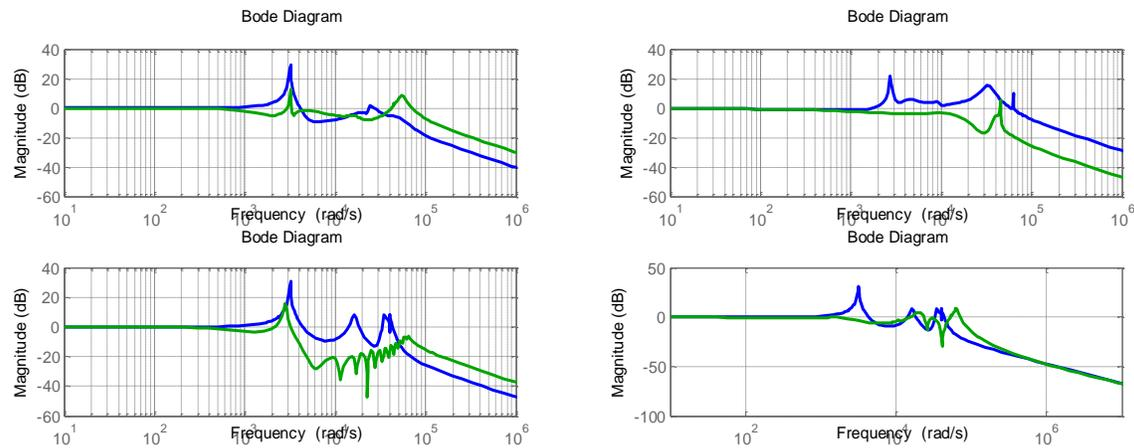
Figure 7- Compensated and un-compensated system frequency responses
