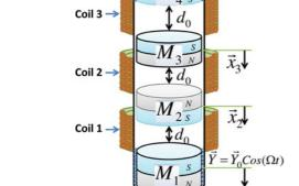
Fig. 5.1 A schematic diagram of the two degree of freedom vibration energy harvester based on magnetic levitation
