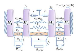
The electrical damping can be expressed as a function of the internal resistance of the coil, the resistance of external load 53 and the electromechanical coupling coefficient. 54
