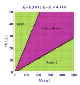
**Fig. 5.3** Variation of the distance separating the eigenfrequencies of the proposed VEH with respect to  $M_1$  and  $M_4$ . Inside the optimal zone,  $f_2 - f_1 < 4.3 Hz$
