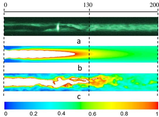
**Fig. 2** Flow visualizations along the mixing tube in the mixed flow regime: **a** laser tomography, **b** subsonic iso-mach (RANS model), **c** subsonic iso-mach (LES model)
