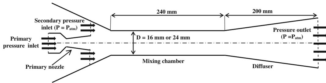
**Fig. 1** Cross-sectional view of the ejector
