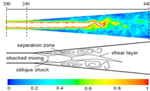
**Fig. 3** Flow visualization along the diffuser in the supersonic flow regime: subsonic iso-mach (LES model) vs. explanatory scheme
