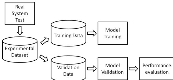
Fig. 4. Framework to apply ANN in system identification.
