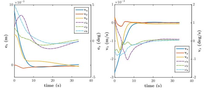
Fig. 6. Positioning task [simulation case]: (left) pose error decay in each DOF ( $e_t$  for translations and  $e_r$  for rotations) and (right) velocity evolution in each DOF ( $v_t$  and  $v_r$  respectively for the translational and rotational components of the robot control velocity screw)
