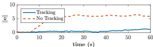
Fig. 13. Evolution of the error in the Shearlet domain with and without tracking.
