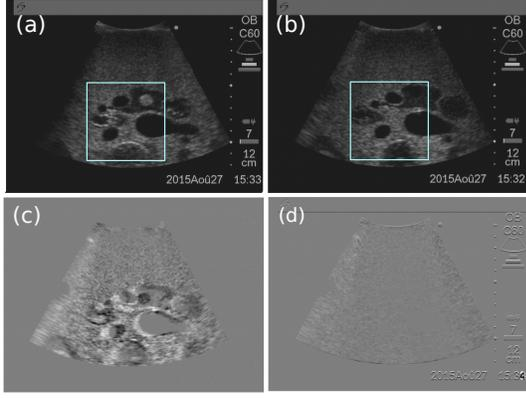
Fig. 8. Image sequence captured during a positioning task: (a) the initial image  $\mathbf{I}(\mathbf{r}_0)$ , (b) the desired image  $\mathbf{I}(\mathbf{r}^*)$ , (c) the difference between the initial and the desired image and (d) the difference between the final and the desired images  $\mathbf{I}_{diff}$ .
