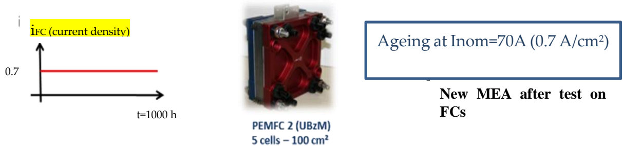
Fig. 7: 2nd long-term test (FCs): 1000 h without current oscillations
