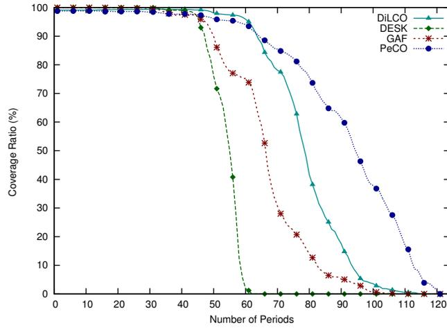
FIGURE 5 – Coverage ratio for 200 deployed nodes.
