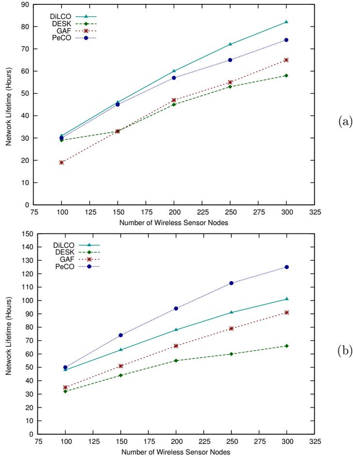
FIGURE 9 – Network Lifetime for (a) *Lifetime<sub>95</sub>* and (b) *Lifetime<sub>50</sub>*.
