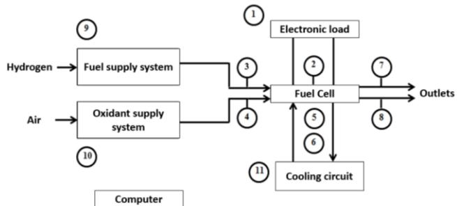
Figure 2: Locations of the different sensors on the test bench
