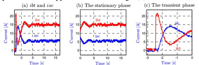
Fig. 6. Current limitation mode in discharge: (a) ibt and isc, (b) the zoom in the stationary phase, (c) the zoom in the transient phase
