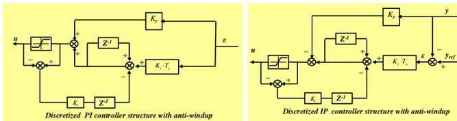
Fig. 3. Discretized PI (left) and IP (right) controllers' structures
