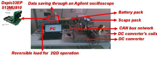
Fig. 1. Electrical network of the system
