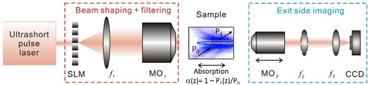
**Figure 1.** Experimental setup for femtosecond Bessel beam shaping and imaging of propagation in fused silica. Beam scanning allows us to reconstruct in three dimensions the fluence distribution inside the sample. Far-field scanning is possible by inserting lens  $f_2$  in the setup. MO: microscope objective. Absorption measurements of the incident beam along the plasma column were deduced from the measured power distribution as indicated.
