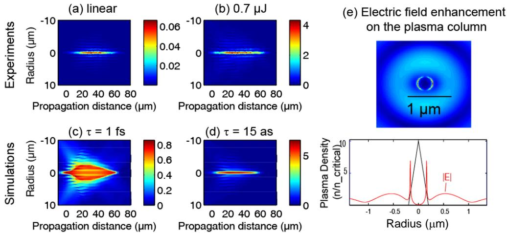
Figure 2. Comparison between experimental fluence maps (a-b) and simulations with nonlinear Schrödinger model (c-d). The unit of fluence used in the colormaps is  $\text{J}/\text{cm}^2$ . (e) Modelling results: Top - transverse distribution of linearly polarized electric field. Bottom - line profile of field is shown in red for conditions of a linear plasma density distribution (black).
