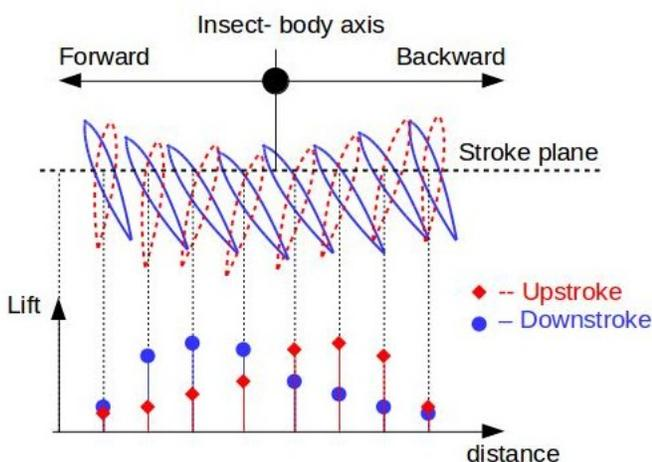
Fig. 5: Insect's lift generation process.
