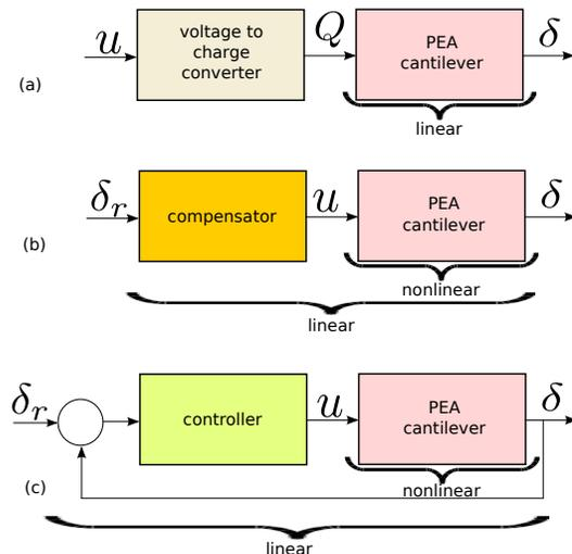
Fig. 3: Displacement control of a PEA actuator. (a) Charge control considering that relationship of the PEA's charge and displacement are linear, (b) Feedforward control structure via an hysteresis/creep compensator, (c) Feedback control structure based on the displacement error
