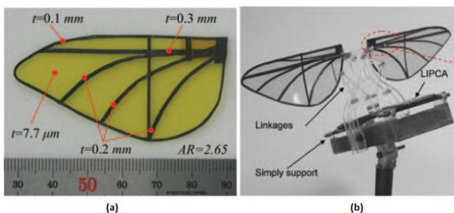
Fig. 9: (a) Artificial Hawkmoth wing; (b) Fully assembled flapping system [64].
