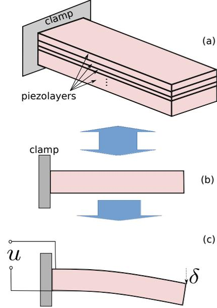
Fig. 1: A piezoelectric cantilevered actuator. (a) Isometric scheme depicting the PEA's piezolayers, (b) Side view of a PEA, (c) bending displacement resulting as a result of the application of an input voltage  $u$
