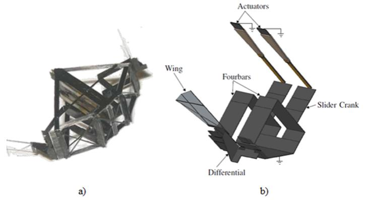
Fig. 6: (a) Current Micromechanical Flying Insect (MFI) design (4DOF); (b) Flying Insect Thorax [57].
