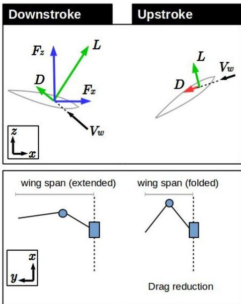
Fig. 4: Avian's lift generation process.
