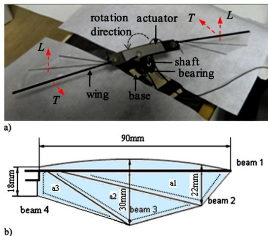
Fig. 8: (a) The proposed configuration; (b) Geometric dimensions of the flapping wing. [60].
