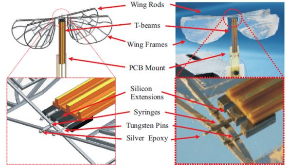
Fig. 7: Conceptual design of the Penn State flapping system (left), four winged piezoelectric flapping system device (right) [2].
