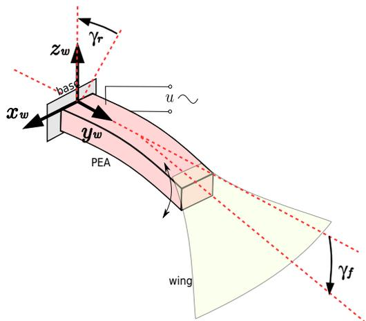
Fig. 10: Perspective Piezowing: the PEA actuates directly to flap microrobot's wing. The flapping angle and wing's lift attitude respectively stand for  $\gamma_f$  and  $\gamma_r$ . The latter angle is generated by a PEA-based joint located at Piezowing's base.
