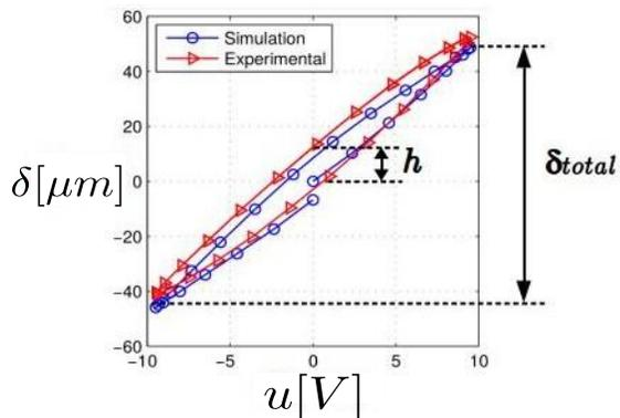
Fig. 2: Curve depicting the non-linear displacement behavior of a PEA.
