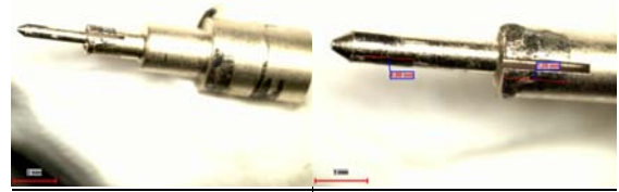
Fig. 14. Optical observation of the fretting scars on the connector tested at D^* = \pm 45\mu\text{m} , N = 15 \times 10^6 cycles, f = 100\text{Hz} .
