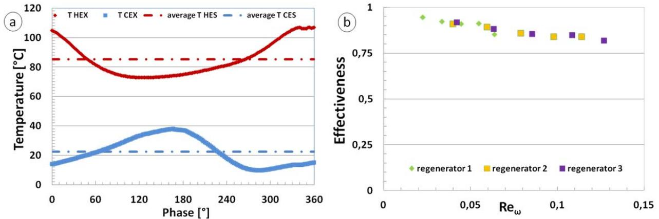
**Figure.6** Example of the evolution of the temperature (a) for a period of a 5.7 Hz flow oscillating at each regenerator extremity ( $\epsilon = 30\%$ ,  $D_h = 0,178$  mm,  $L = 60$  mm,  $T_{HEX} = 79^\circ\text{C}$ ,  $T_{CEX} = 12^\circ\text{C}$ ) and evolution of the effectiveness (b) versus oscillating flow Reynolds number  $Re_\omega$  in the different regenerators.
