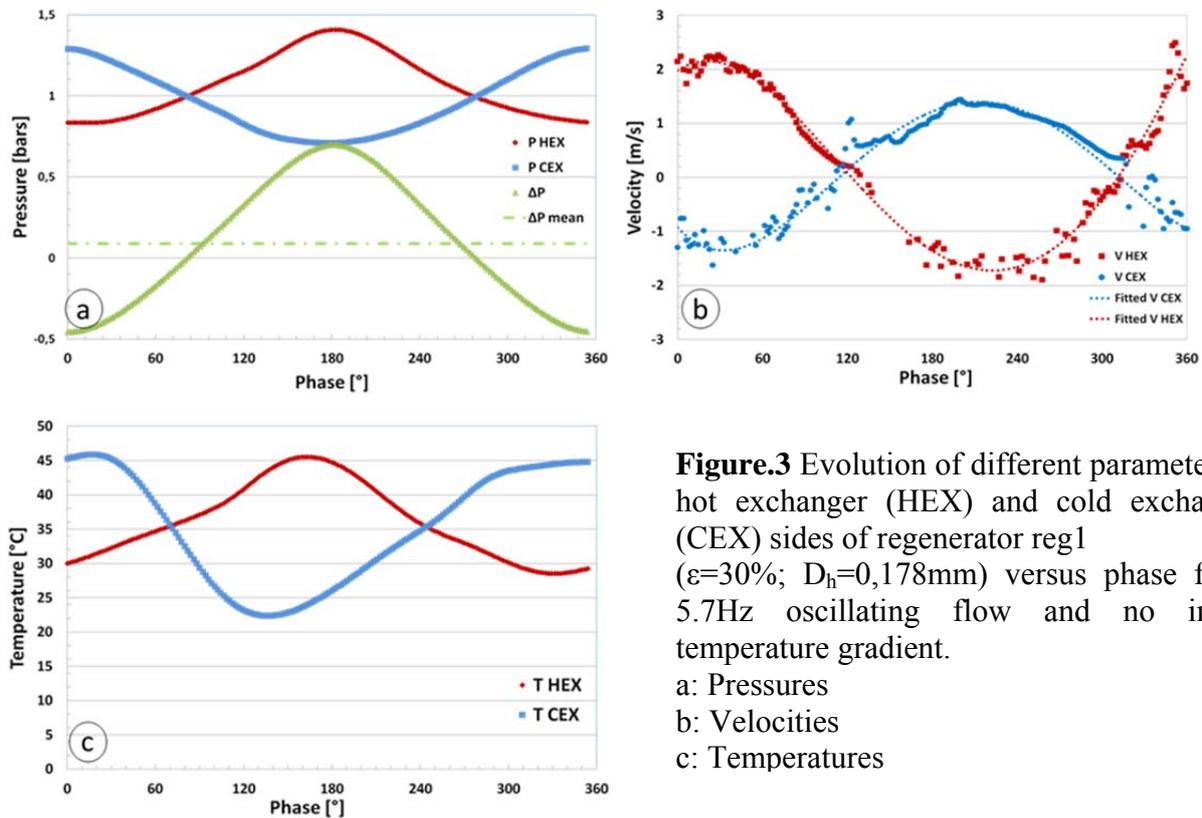
**Figure.3** Evolution of different parameters at hot exchanger (HEX) and cold exchanger (CEX) sides of regenerator reg1 ( $\epsilon=30\%$ ;  $D_h=0,178$ mm) versus phase for a 5.7Hz oscillating flow and no initial temperature gradient.
