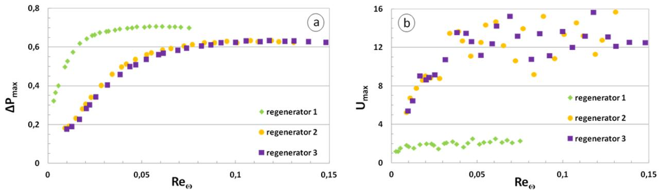
**Figure.4** Evolutions of the maximum pressure drop (left) and the maximum velocities (right). Experiments have been conducted for reg1 ( $\epsilon=30\%$ ;  $D_h=0,178$  mm), reg2 ( $\epsilon=35\%$ ;  $D_h=0,237$  mm), reg3 ( $\epsilon=40\%$ ;  $D_h=0,250$  mm) and a wide range of frequencies (0.2 to 5.8 Hz).
