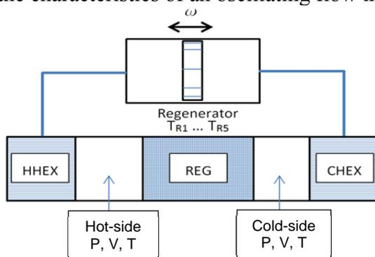
**Figure.1** Scheme of the experimental bench for regenerator test
