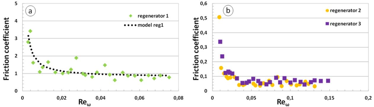
**Figure.5** Evolutions of the friction factors for reg1 (a), reg2 and reg3 (b). Experiments have been conducted on a 60 mm long regenerator for 3 different porosities (30, 35 and 40%) and a wide range of frequencies (0.2 to 5.8 Hz).
