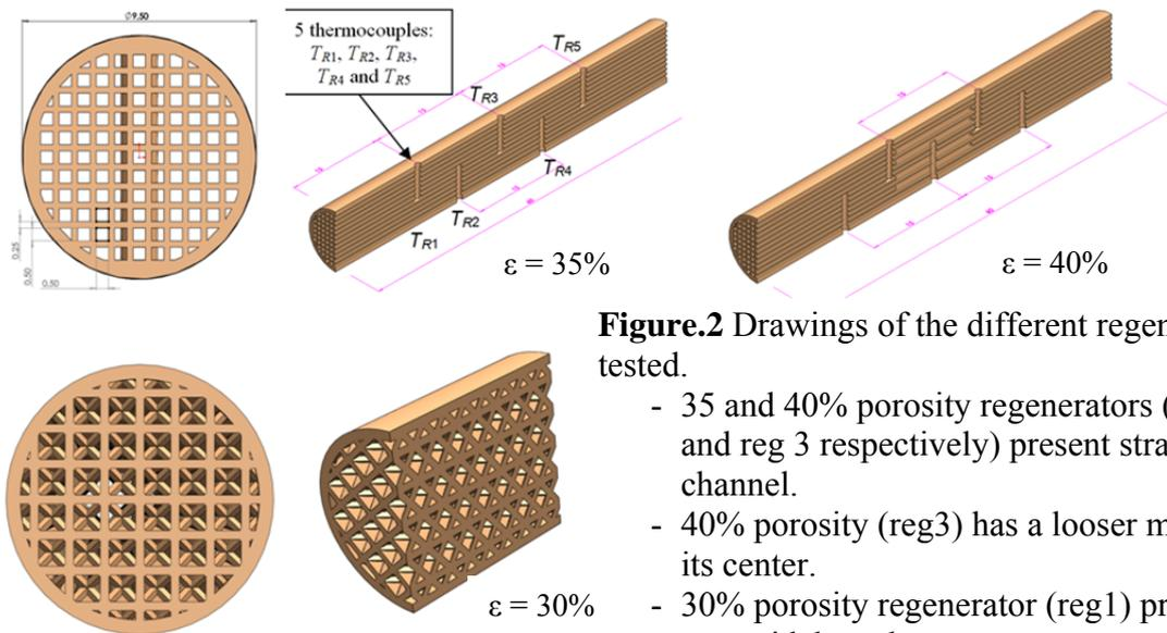
**Figure.2** Drawings of the different regenerators tested.
