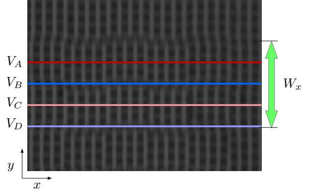
Figure 4: An example of selection of four horizontal lines used to find the best working area. The image is averaged vertically beforehand. Each line is chosen \tilde{W}_x/4 away from the previous line.
