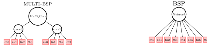
Fig. 4 The difference between the MULTI-BSP and BSP models for a multicore architecture.
