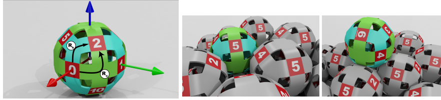
Fig. 6 A catom with two methods of rotation: R_h in the hexagonal area and possible but not the other one. R_o in the octagonal area.
