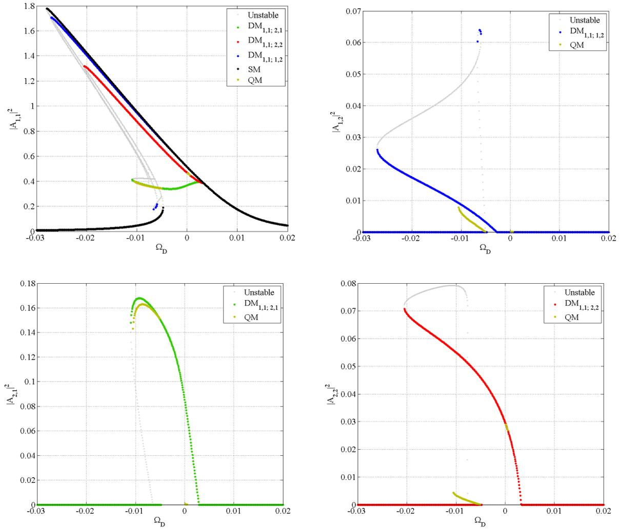
Figure 5: Response intensities of  $2 \times 2$  weakly coupled oscillators under harmonic base external excitation as a function of the detuning parameter  $\Omega_D$ , for the fourth set of design parameters listed in table 1.
