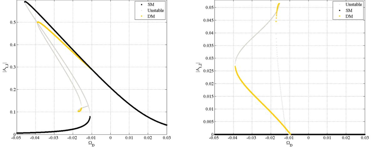
Figure 2: Response intensities of two weakly coupled oscillators under harmonic base external excitation as a function of the detuning parameter  $\Omega_D$ , for the first set of design parameters listed in table 1.
