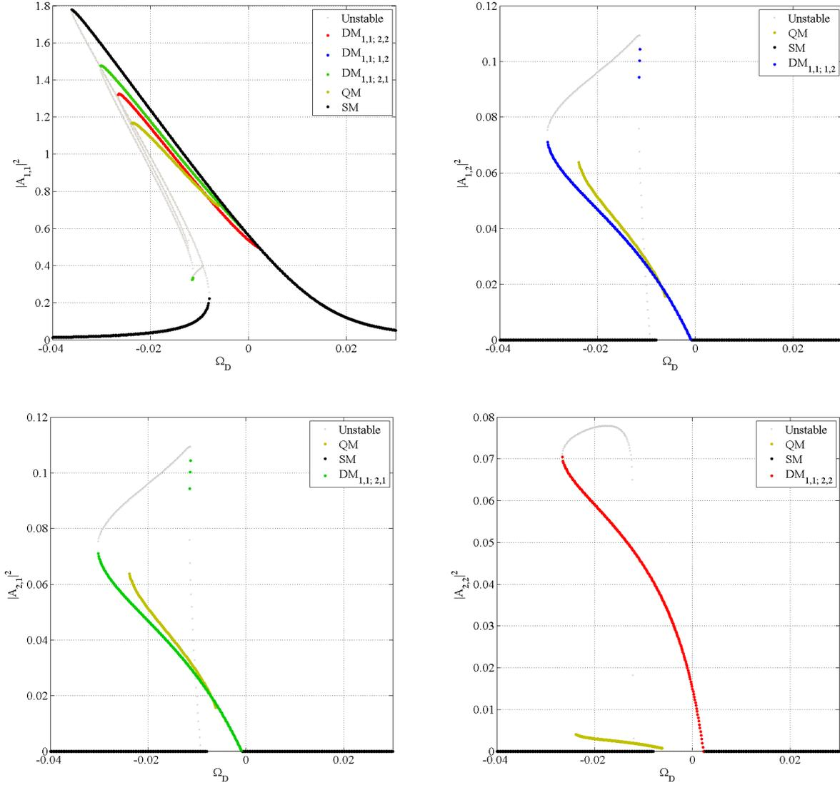
Figure 3: Response intensities of  $2 \times 2$  weakly coupled oscillators under harmonic base external excitation as a function of the detuning parameter  $\Omega_D$ , for the second set of design parameters listed in table 1.
