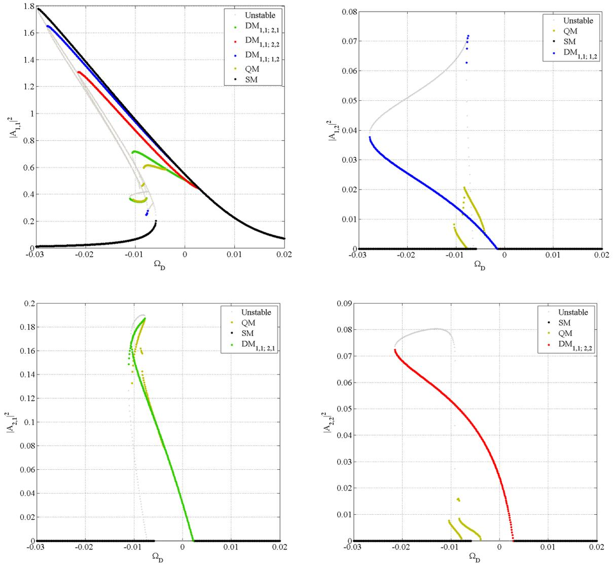
Figure 4: Response intensities of  $2 \times 2$  weakly coupled oscillators under harmonic base external excitation as a function of the detuning parameter  $\Omega_D$ , for the third set of design parameters listed in table 1.
