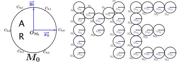
Fig. 1. Shape form by circular 2D Mems arrange in a honeycomb grid (to form M) and an orthogonal grid (to form E) and a highlight of a Mems with it's landmarks and surface connectors
