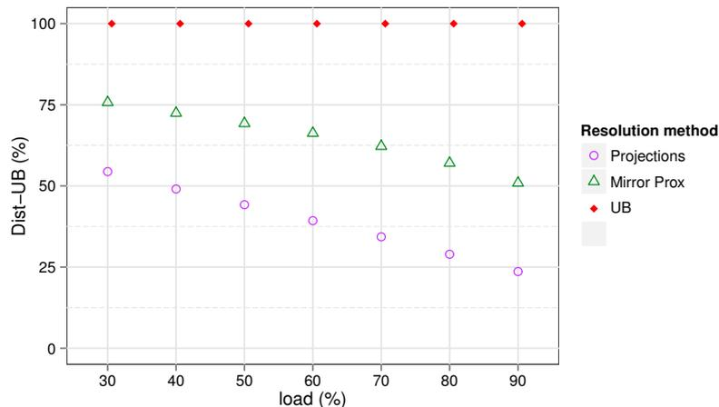
Figure 2: Distance to the upper bound UB of production horizons reached with each convex resolution method for different load demand values –  $m = 25$  machines
