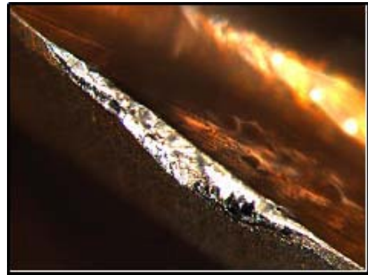
Fig. 5: Flank tool wear after 320 cuts
