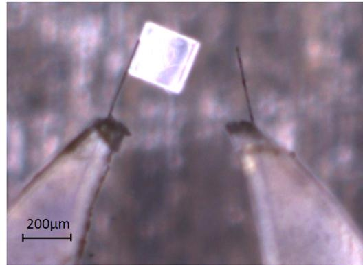
Fig. 1: Illustration of the adhesion effect: only one finger is required to have a stable grasp
