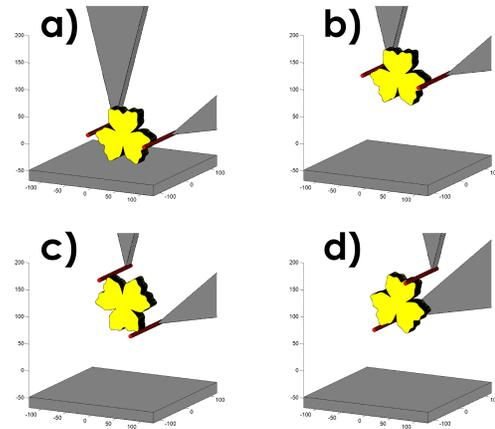
Fig. 7: Images sequence describing the clockwise trajectory generated by the planner for a  $130^\circ$  rotation considering adhesion phenomena.
