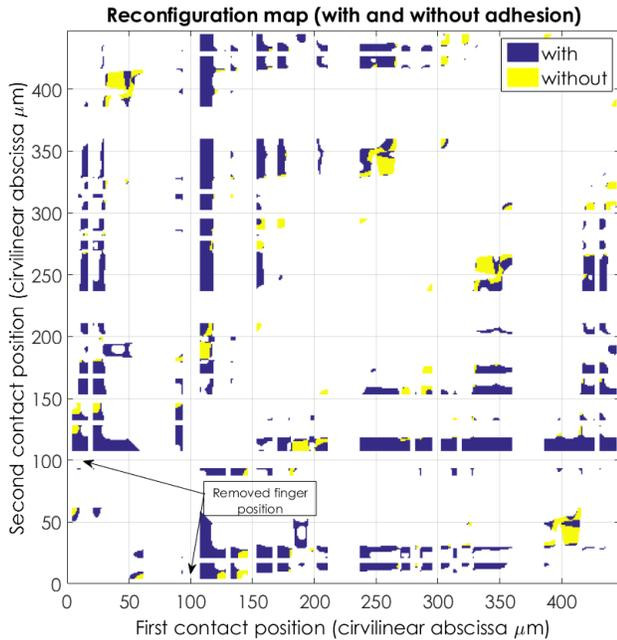
Fig. 6: Representation of the set  $D_3$  (reconfiguration map) with and without adhesion on an arbitrary shaped object depicted in Fig.7.
