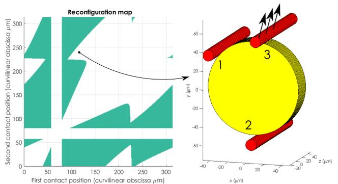
Fig. 4: Representation of the set  $D_3$  (reconfiguration map) for an assigned location of the third contact considering adhesion (sticky behavior,  $\forall i, w_{po_i} \neq 0$ ).
