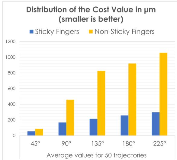
Fig. 9: Chart representing the distribution of the trajectory cost value for various rotation amplitudes and condition of use. For each rotation amplitude and each case fifty rotations were generated.
