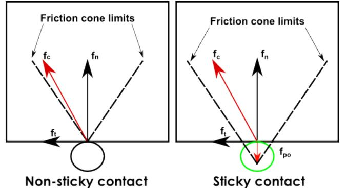
Fig. 2: Side view illustrating the impact of adhesion on the friction cone.
