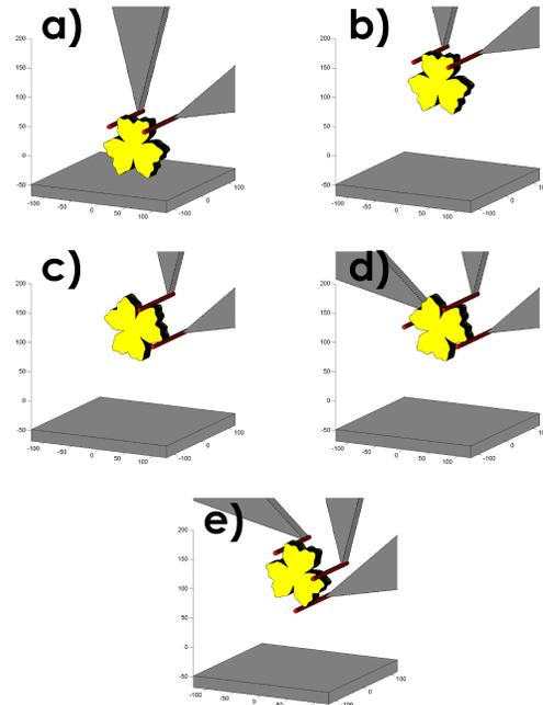
Fig. 8: Images sequence describing the clockwise trajectory generated by the planner for a  $130^\circ$  rotation without considering adhesion phenomena.
