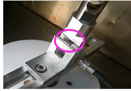
Fig. 3. Three–points bending experiment of a packaged chip (inside the ellipse mark).
