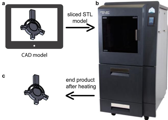
Fig. 2. 3D printing steps. (a): CAD design and data model generation. (b): 3D printing machine. (c): end product after heating.
