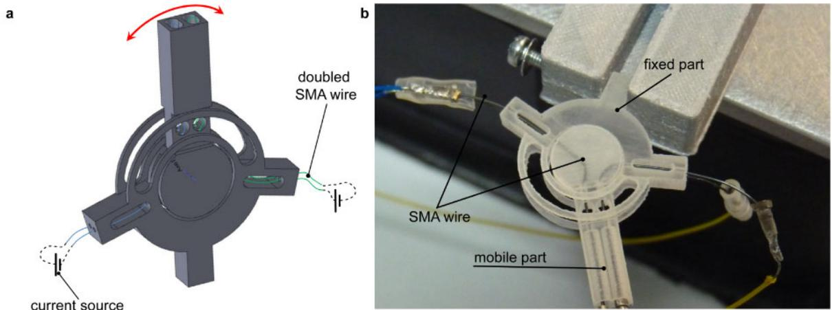
Fig. 4. Functionalization of the articulation by using SMA wire. (a): SMA wires distribution. (b): realized articulation equipped with SMA wires.
