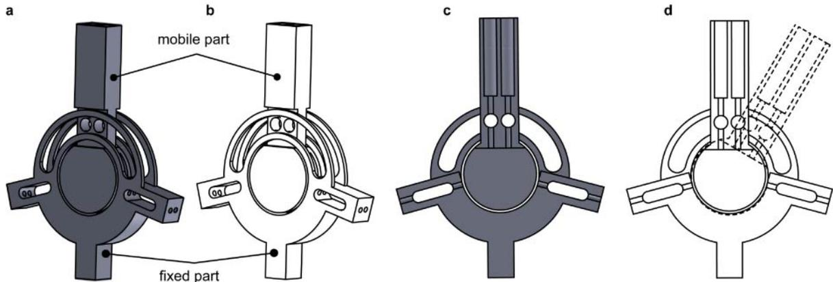
Fig. 1. Pivot articulation design. (a): CAD model of the articulation link. (b): wire representation of the CAD model. (c) and (d): cross section of the CAD model showing the expected grooves and holes allowing to introduce the SMA wire.
