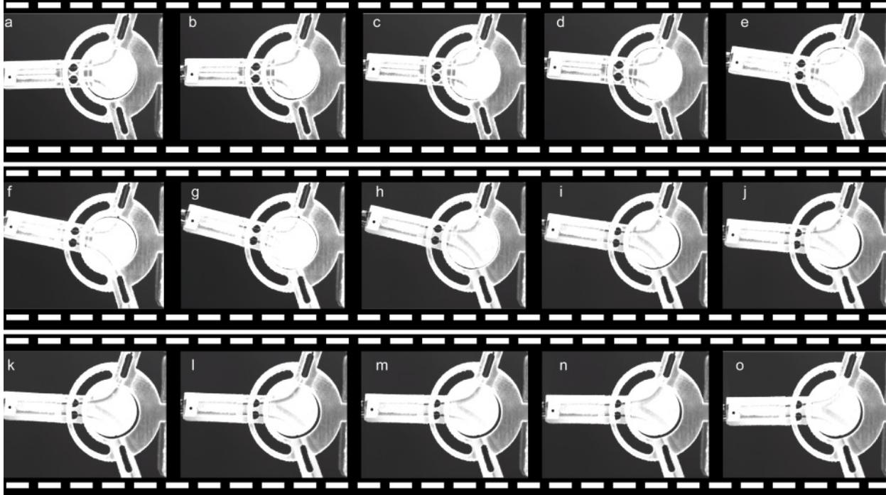
Fig. 6. Visual feedback sequence of the displacement of the articulation according to the actuated wire. (a to h): positive displacement caused by the actuation of the wire-1. (i to o): negative displacement caused by the actuation of the wire-2.
