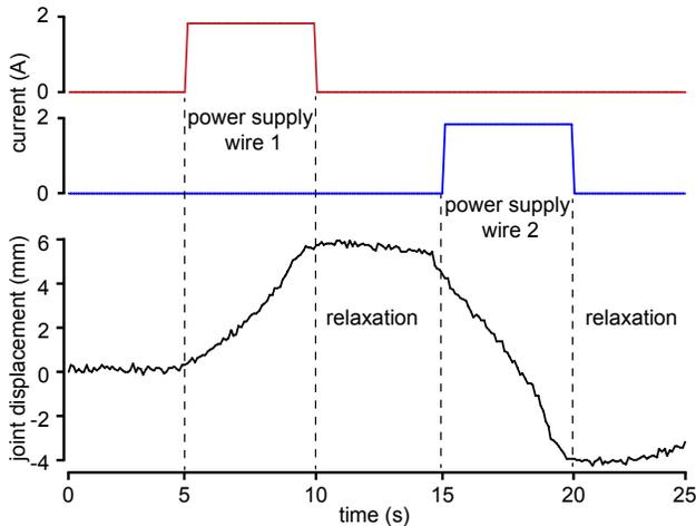
Fig. 5. Displacement of the extremity of the mobile part of the joint along Y axis according to time. The positive displacement is generated when wire-1 is actuated while the negative displacement comes with the actuation of wire-2. For each case, a square current impulse with an amplitude of 2 A and a width of 5 s is used.
