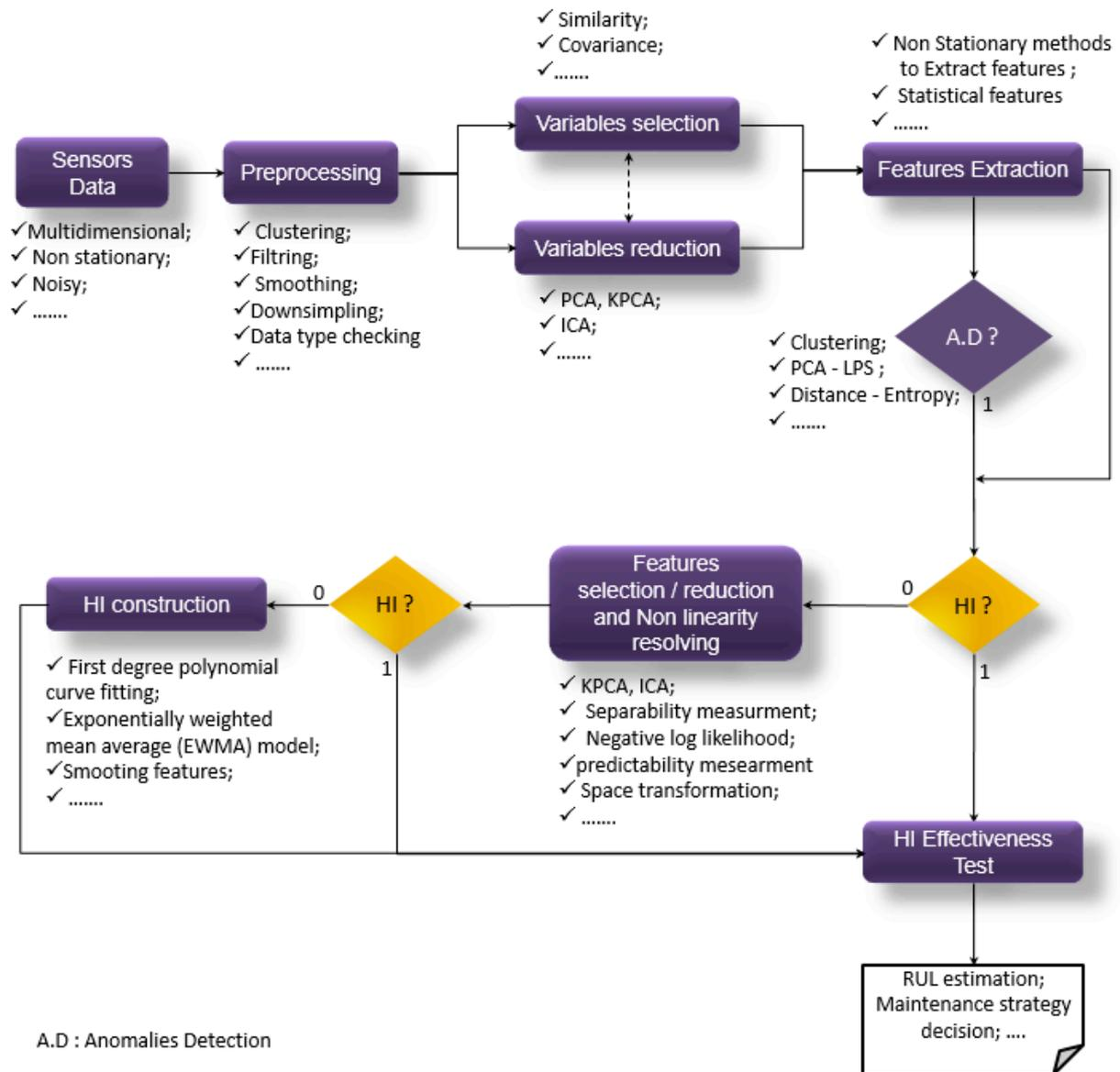
Figure 2. Proposed approach diagram for HI construction.
