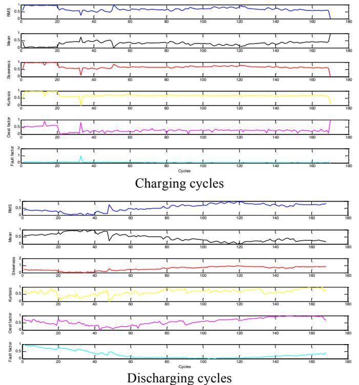
Figure 6: Time domain features extracted from first Principal Component of selected variables.
