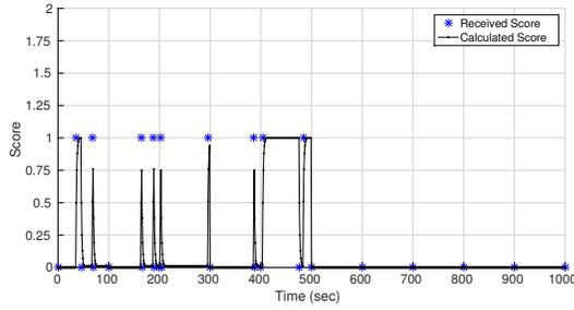
**Figure 4: The scores of the received measurements from the Heart Rate biosensor node and the calculated up-to-date score by the coordinator over 10 rounds.**
