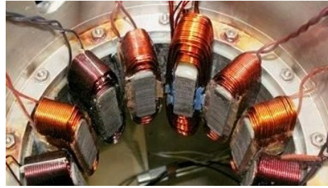
(b): on-tooth SRM windings
