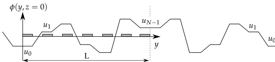
**Figure 3.** Transcription of the boundary conditions to the potential approximate on the electrode plane. The non-flux condition on the lateral wall is seen as a symmetry. The potential between each pair of electrode is approximated by a linear function.
