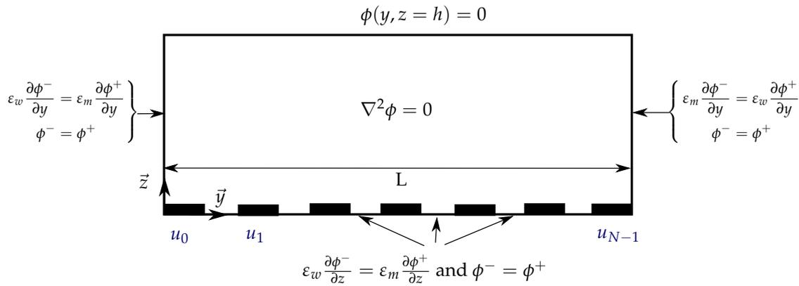
**Figure 2.** Schematic representation of the boundary conditions determining the electric potential above an array of electrodes.  $\phi^+$  and  $\phi^-$  are the electric potentials on each side of the boundary.  $\epsilon_m$  is the permittivity of the fluid in the channel and  $\epsilon_w$  is the permittivity of the wall.
