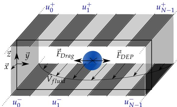
**Figure 1.** Sketch of the proposed sorting stage, based on electrode arrays, integrated in a fluidic chip. The cells flow through a channel due to the fluid motion. The lateral position of the cells is controlled by the electric potential applied on each electrode at the top and the bottom of the channel. Moving the cell along the  $y$  axis enables to collect them in different reservoirs to sort them.
