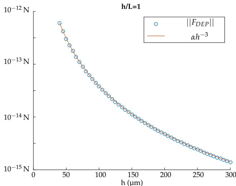
**Figure 8.** Example of the analysis of the impact of one geometrical parameters on the DEP force: Influence of the height  $h$  of the channel, for  $h/L = 1$ . The plotted force values correspond to the mean value of the quadratic norm of the dielectrophoretic force on the segment ( $y \in [L/3; 2L/3], z = 0$ ). The number of electrodes is  $N^+ = N^- = 8$  and the voltage applied on them is detailed in Figure 5.
