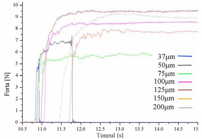
Fig. 16. The maximum force and response time to the nominal current value for different wire diameters.
