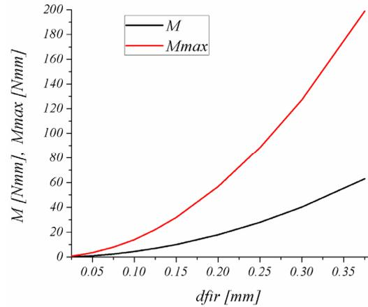
Fig. 7a. The variation of the torque depending on the SMA wire diameter.
