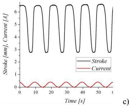
Fig. 11. Applied current and related displacement output variation of the MAMF-03-00 actuator of 150 $\mu$ m diameter, for a sine wave of frequency 0.01Hz(a), 0.05Hz(b), 0.5Hz(c).
