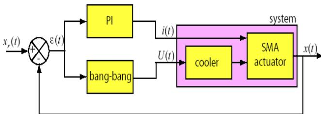
Fig. 15. The block diagram of the closed-loop control.
