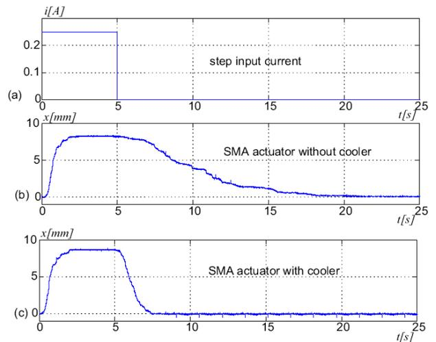
Fig. 14. (a) Step input current applied to the actuator, (b) Step response of the actuator without cooler, (c) Step response of the actuator with cooler.
