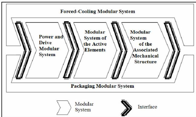
Fig. 1. The modular structure of the SMA actuators.
