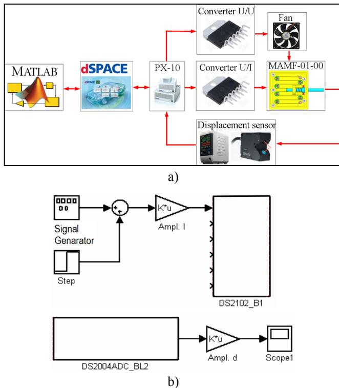
Fig. 9. a) The block diagram of the linear actuators testing workbench. b) Simulink model.
