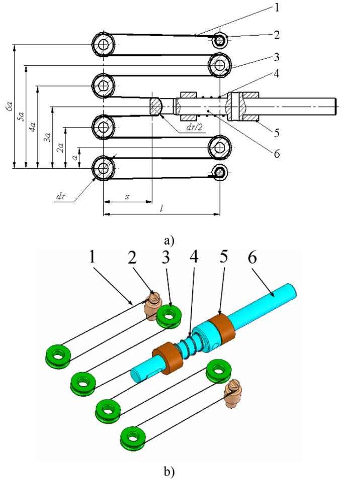
Fig. 2. The mechanical structure of the linear actuators.
