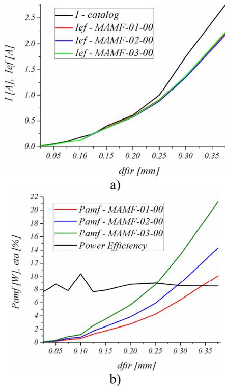
Fig. 4. The load current and the power dissipation on different SMA wires diameters.
