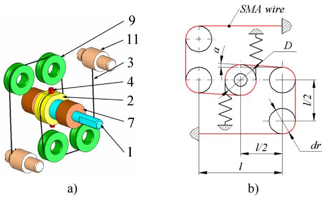
Fig. 6. The operation principle of the rotary SMA actuators.
