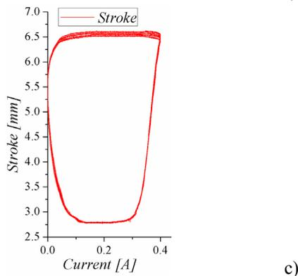
Fig. 12. Current - displacement characteristics of the MAMF-03-00 actuator, for a sine signal at 0.01Hz (a), 0.05Hz (b), 0.5Hz (c) frequency and 150 $\mu$ m diameter of the SMA wire.
