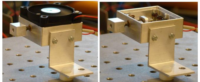
Fig. 10. SMA linear actuator with and without fan cooling.
