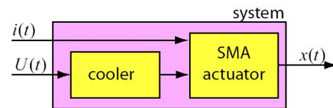
Fig. 13b. The DISO model of the SMA actuator with cooler.
