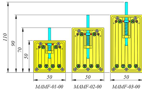
Fig. 3b. The three linear actuators and their overall dimensions.
