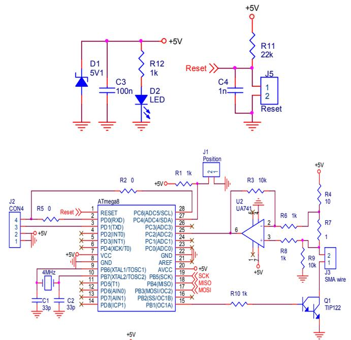
Fig. 5. The electronic schematic of the linear actuator.
