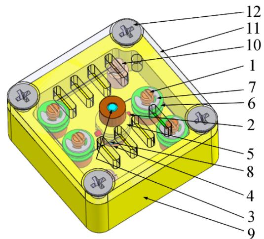
Fig. 7b. 3D mechanical model of the designed rotary SMA actuator.
