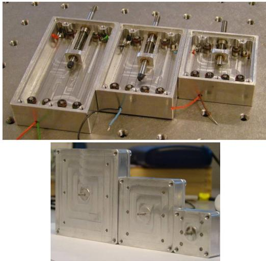
Fig. 8. Pictures representing the developed prototypes of linear and rotary SMA actuators.
