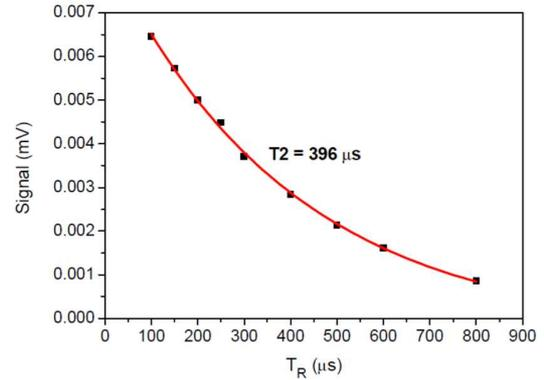
Fig. 5. Fringe amplitude versus the free-evolution time  $T_R$ .
