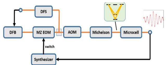
Fig. 1. Schematic of the Cs CPT clock. DFS: Dual-frequency Doppler-free spectroscopy.
