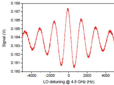
Fig. 3. Ramsey-CPT fringes detected in a Cs—Ne microfabricated cell.
