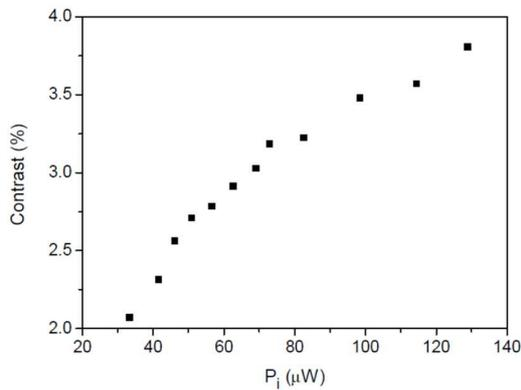
Fig. 4. Fringe contrast versus the incident laser power. Experimental parameters are  $T_R = 300 \mu\text{s}$ ,  $T_b = 400 \mu\text{s}$ .
