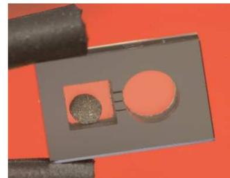
Fig. 2. Photograph of a Cs-Ne microfabricated cell.
