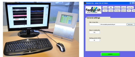
Figure 10. (left) Labview VI for raw signal visualization and (right) the graphical user interface to set the optional parameters (if required) of the signal processing algorithms.
