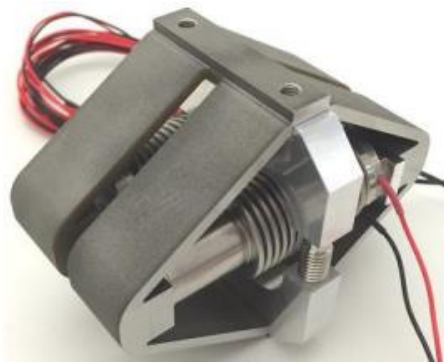
Figure 4: APA95-PTW-MD actuator, from [6]
