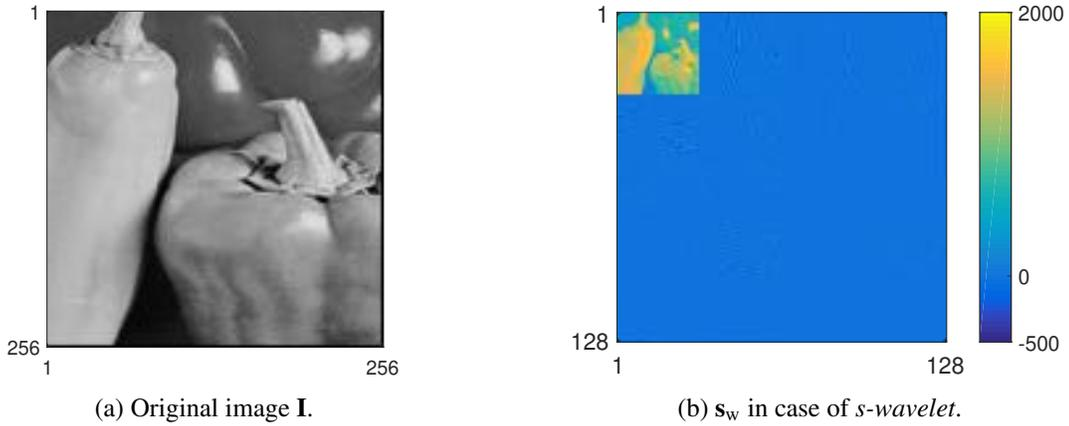
Figure 6: The feature vector  $\mathbf{s}_w$  was obtained by performing a discrete wavelet transform at level 3. The upper left corner in Fig. 6b contains a coarse approximation of the original image of size  $32 \times 32$ . The remaining pixels correspond to detail coefficients at the second and third stage of decomposition. Note that the high-frequency detail coefficients from the first stage of decomposition were omitted.
