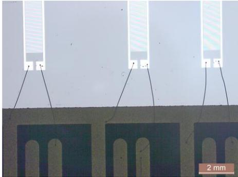
Figure 3. IDT patterns on LiNbO<sub>3</sub> wafer connected to printed circuits by wirebonding.
