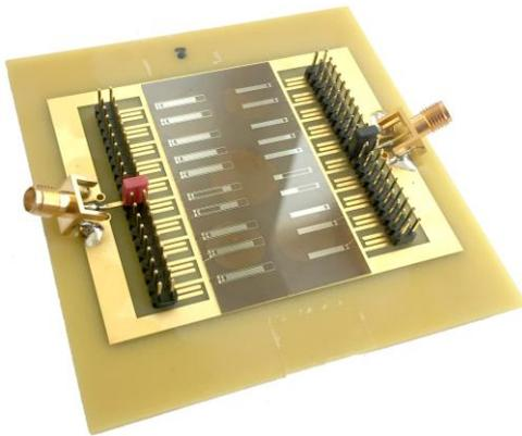
Figure 4. Photography of the test ready final device with in/out SMA connectors.
