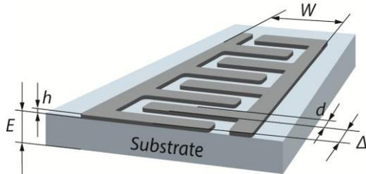
Figure 1. 3D perspective view of the SAW device.
