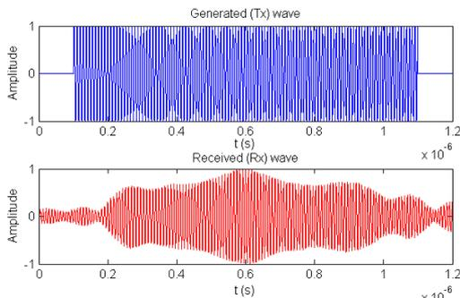
Figure 5. Temporal spectrum of transmitted (bleu) and received (red) acoustic wave. The signal amplitudes are normalized.
