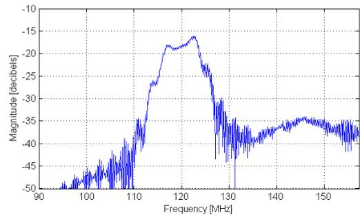
Figure 6. The S<sub>21</sub> frequency response of the IDT (120MHz central frequency and 10MHz Bandwidth).
