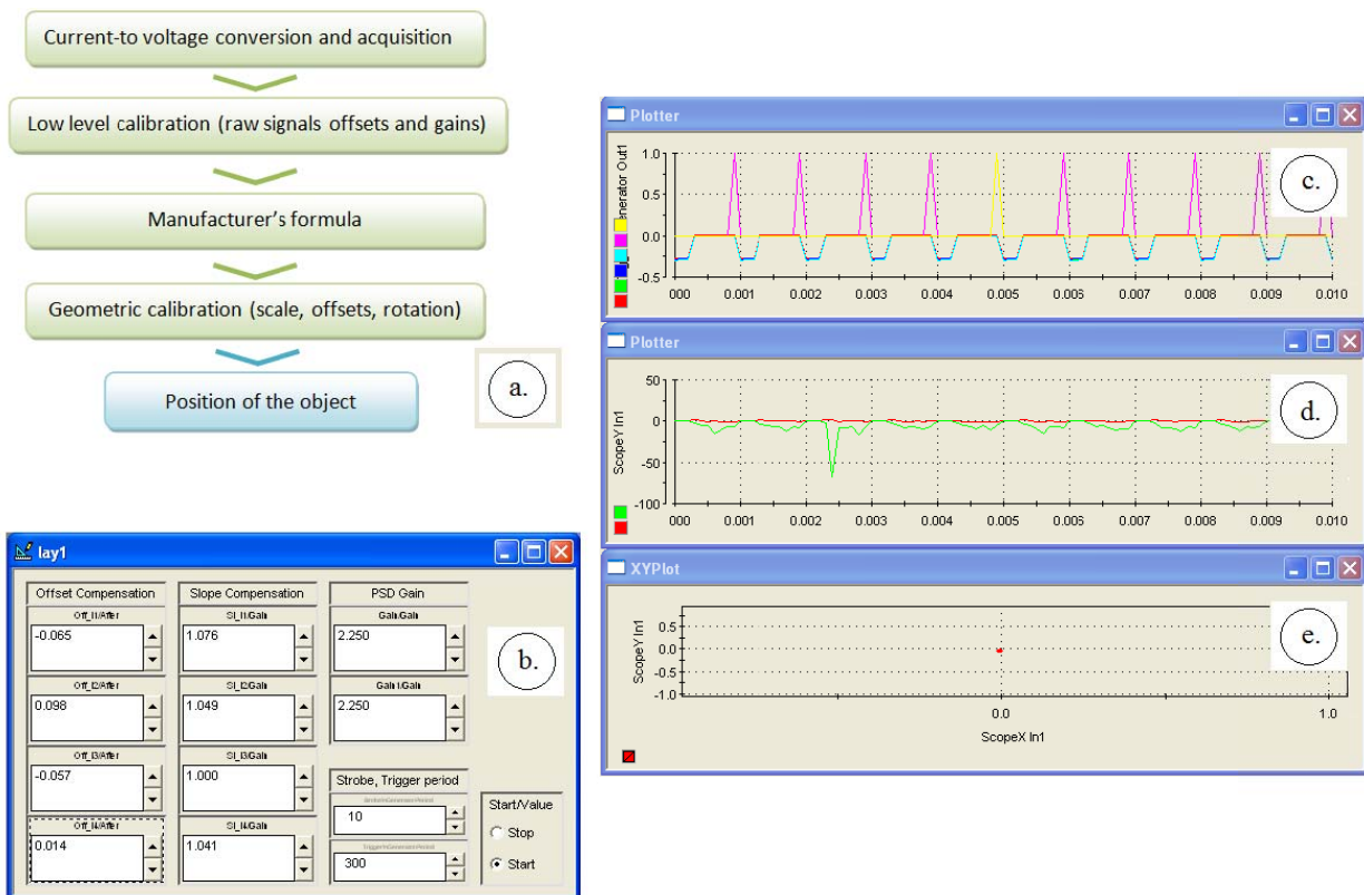
Figure 5. The calibration procedure: (a) shows the conversion sequence block diagram (b) shows the initial calibration window of the four raw PSD signals, (c) shows the raw plot of the four PSD signals as well as the stroboscopic digital impulse train (d) contains the raw x & y charts and (e) is the final x - y graph of filtered values (the PSD spot).
