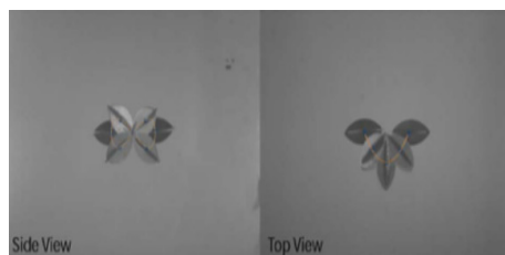
(a) The top and side view of the OctoMag's micro-robot controlled to follow an \infty -shaped trajectory. The micro-robot's orientation is kept toward the center of the sphere.
