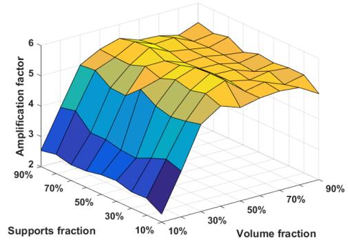
Fig. 5. Estimated amplification factor of designs. Volume and supports fraction ranged from 10% to 90%.
