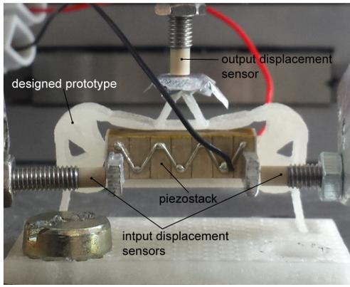
Fig. 8. Experimental bench picture.
