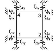
Fig. 2. Support modeling where each node have springs attached in X and Y direction.
