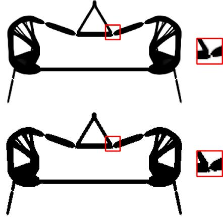
Fig. 7. Selected structure before (up) and after (down) post processing. On the right a zoom on one node hinge before and after post processing.
