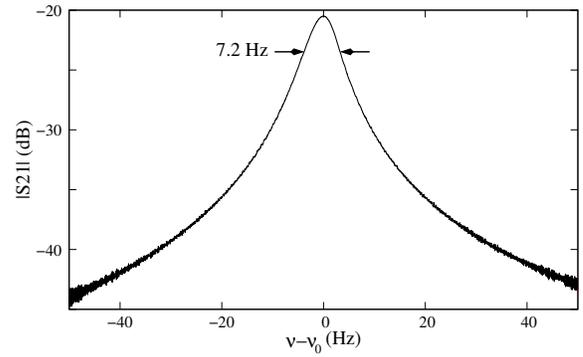
Fig. 7. Transmission resonator response around the resonance frequency  $\nu_0 \approx 10$  GHz.
