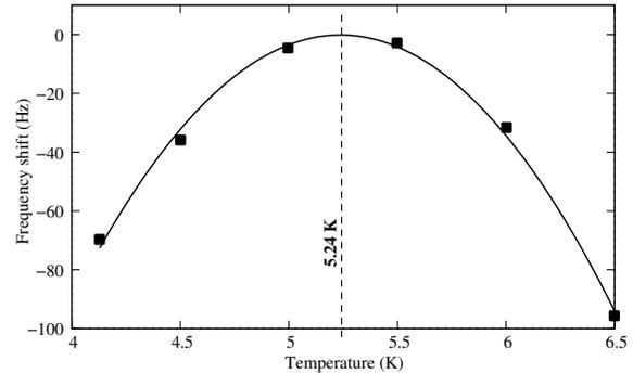
Fig. 8. Resonator frequency evolution around the turnover temperature.
