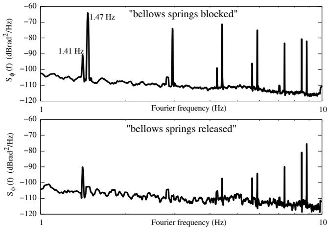
Fig. 9. Upper curve: Phase noise when the bellows springs are blocked. Lower curve: bellows springs released.
