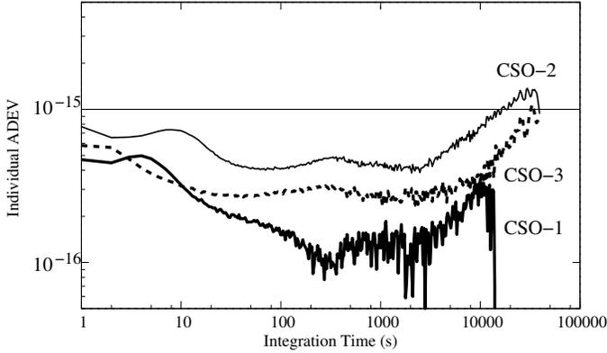
Fig. 2. The three individual ADEV obtained from the 3-cornered-hat method.
