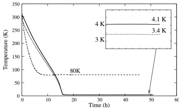
Fig. 6. Temperatures evolution during cool-down. Resonator temperature (bold line), 2<sup>nd</sup>-stage shield temperature (dotted line), 1<sup>st</sup> stage shield temperature (dashed line).
