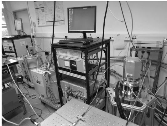
Fig. 1. The three CSOs of the OSCILLATOR-IMP platform.
