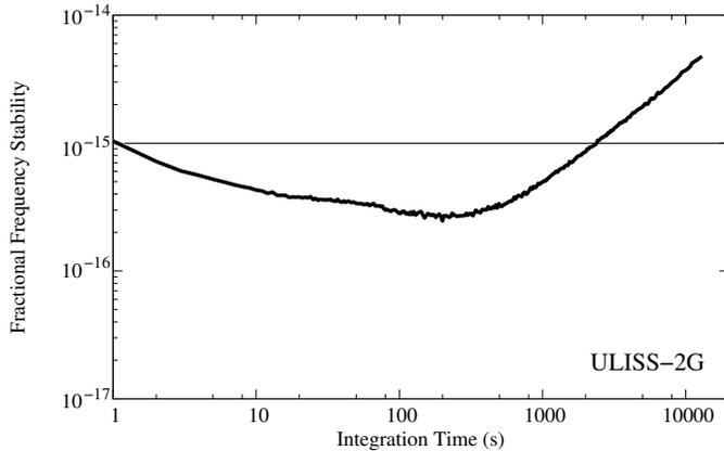
Fig. 10. Fractional frequency stability of the 3 kW prototype evaluated using the three-cornered-hat-method with two ultra-stable 6 kW CSOs used as references [12].
