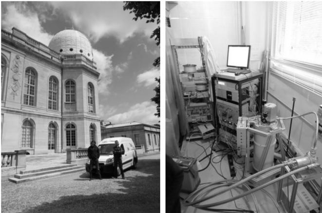
Fig. 3. ULISS in SYRTE, where it was used as flywheel oscillator to run the fountain atomic clock.
