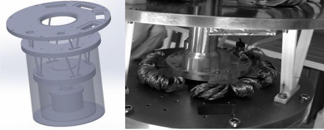
Fig. 5. Internal 3D view of the cryostat and picture of the 2<sup>nd</sup> stage suspension.
