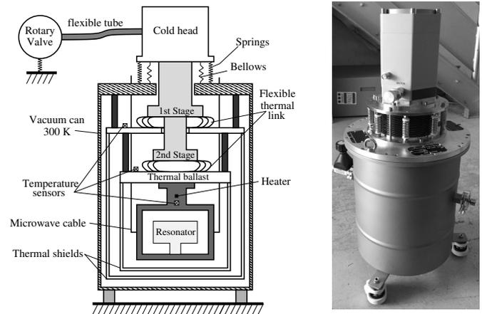
Fig. 4. CSO cryostat: design overview (left), picture of the prototype (right). The rotary valve is located remotely from the cryostat.
