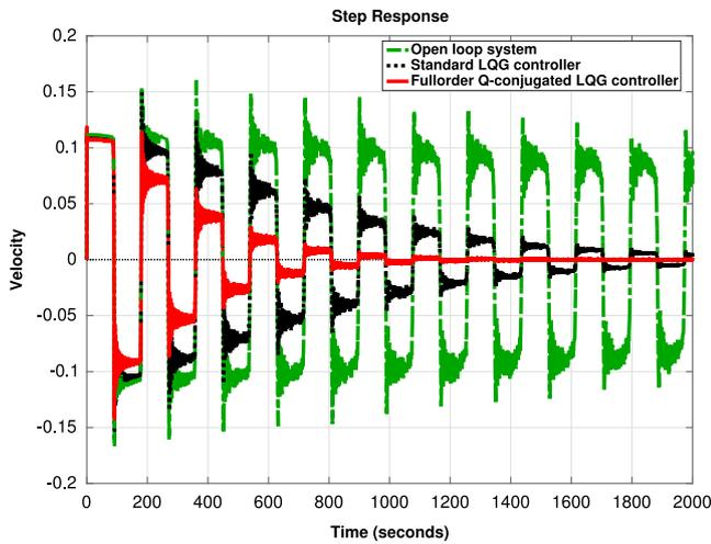
Fig. 1. Step responses of the closed loop (full order) system with standard (full order) LQG controller and (full order) Q-conjugated LQG controller.
