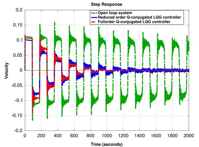
Fig. 3. Step responses of the closed loop (full order) systems with Q-conjugated full order and reduced order controllers.
