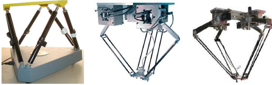
Fig. 1. From left to right: the Gough-Stewart platform (Institut Pascal), the H4 and the Par4 robots (LIRMM).
