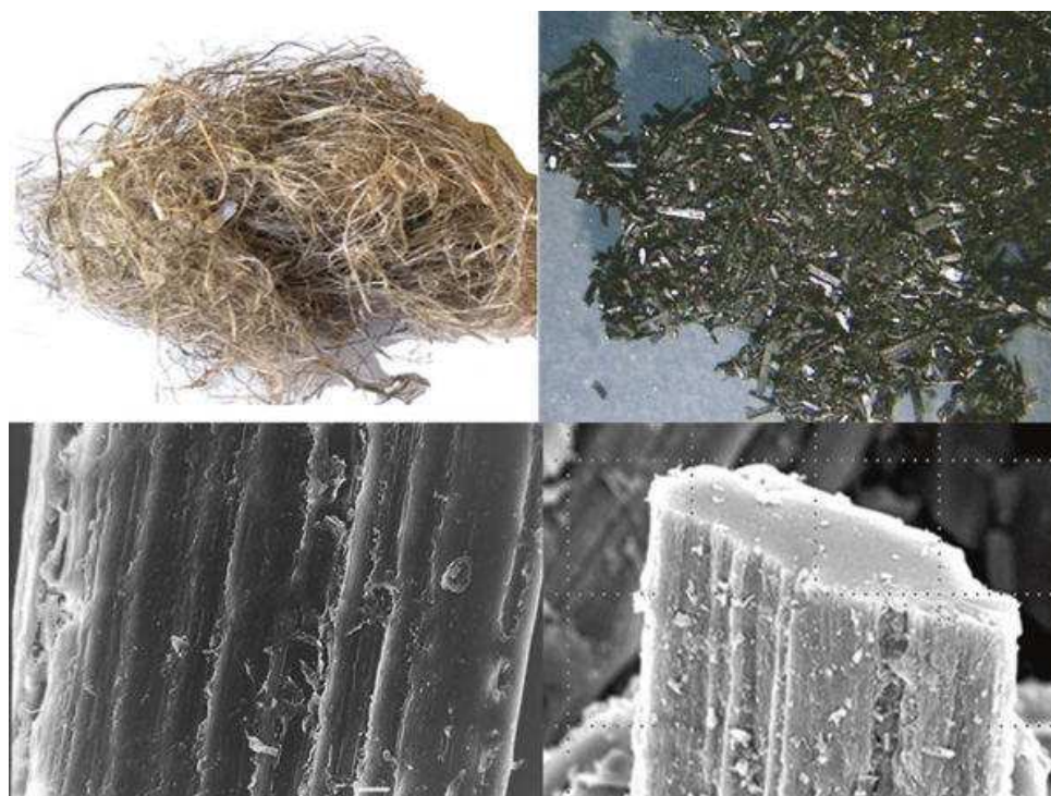
Fig. 1.10 Short hemp fibers before (left) and after (right) carbonization. (Adapted from Vukčević et al. 2015)
