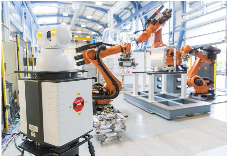
Fig. 6. Nikon laser radar MV331 in the FA 3 D
