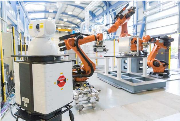
Fig. 7. Nikon laser radar MV331 in the FA<sup>3</sup>D
