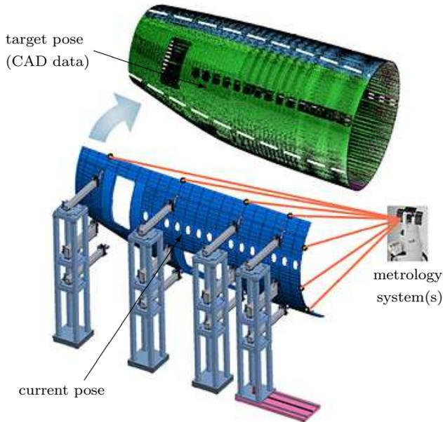
Fig. 1. Measurement Assisted Assembly conceptual model as introduced by Meffert et al. (2012) for the *EcoPositioner* developed by Dürr
