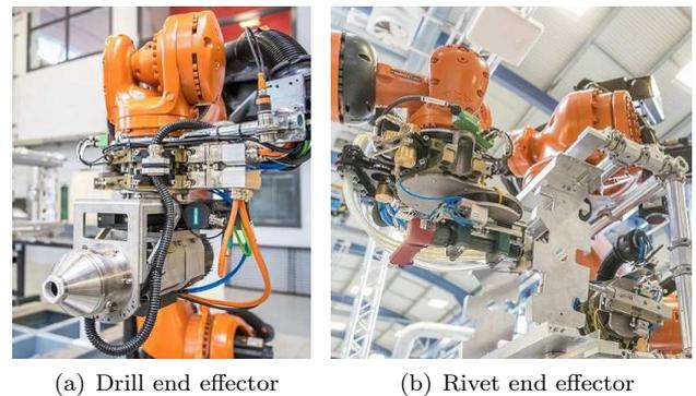
Fig. 5. Drill (on the left) and rivet (on the right) end effectors in the FA<sup>3</sup>D
