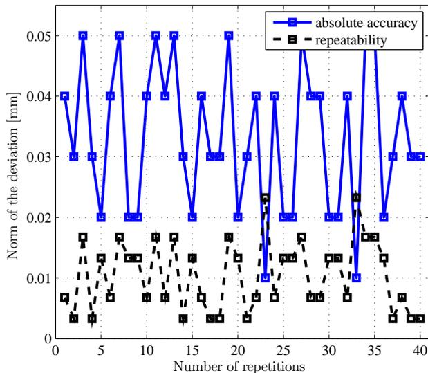
Fig. 10. Absolute accuracy and repeatability performance of the FA<sup>3</sup>D positioning system for a 2400 × 800 mm aircraft component
