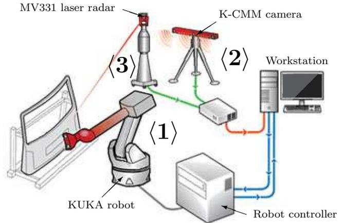
Fig. 9. Diagram of the FA<sup>3</sup>D positioning system
