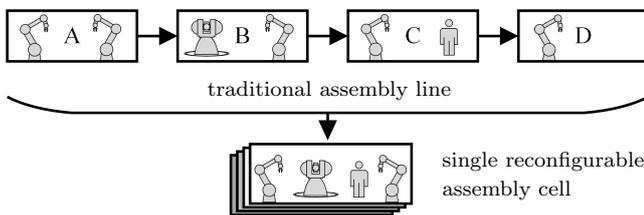
Fig. 2. Compression of an assembly line down to an assembly cell
