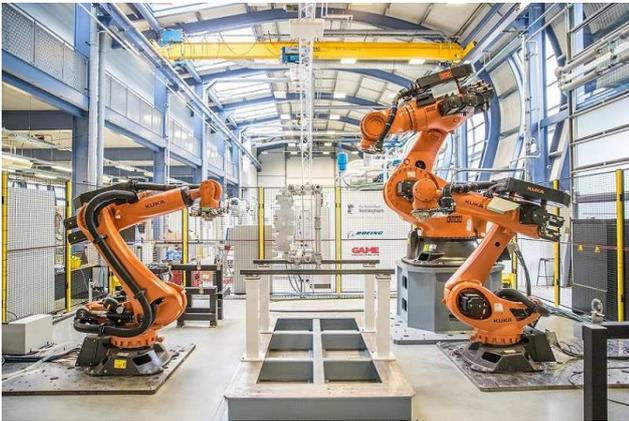
Fig. 4. Reconfigurable assembly cell of the Future Automated Aircraft Assembly Demonstrator developed by the University of Nottingham
