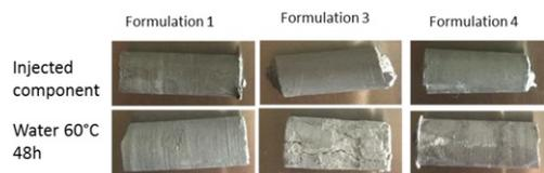
Figure 3 Fig. 3 Images of components before and after water debinding for Formulations 1, 3, and 4.
