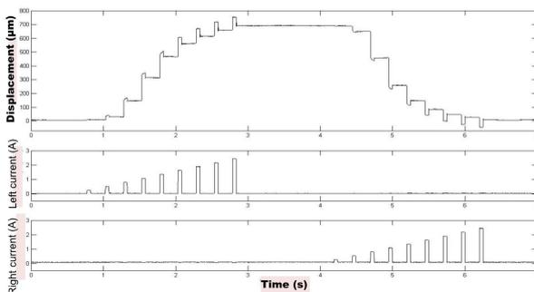
Figure 8: Current pulses control of the MSMA-based actuator.
