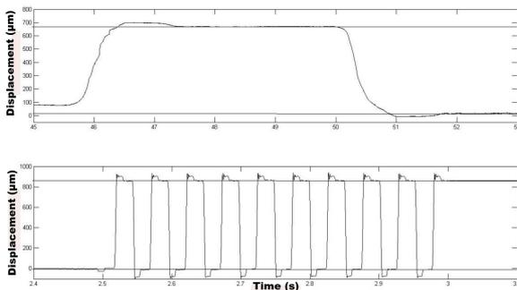
Figure 7: Displacement measurements of the MSMA-based actuator (low and high velocity modes of working).
